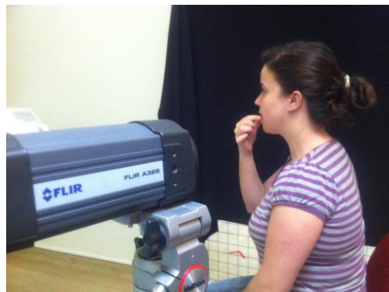
Fig. 3 - Camera Flir A325 capturing thermal images during mastication.
